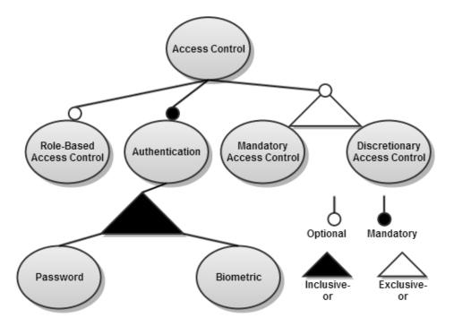
Figure 10.3: Feature Diagram Notation
