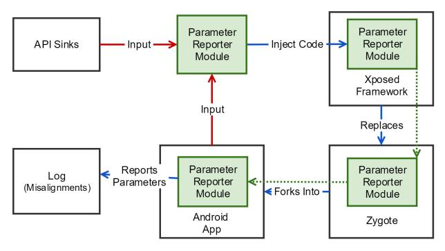
Figure 6.1: Xposed Parameter Reporter Module
