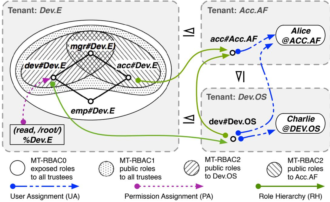
**Figure 3.3:** Example multi-tenant assignments in the out-sourcing case. The differences among the MT-RBAC models are also illustrated in terms of  $E$ 's exposed roles.
