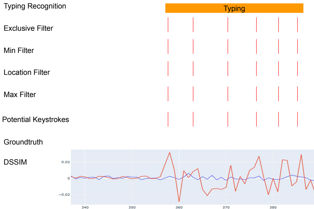
Figure 2.6: An example of our typing activity detection heuristics being applied on potential keystrokes, which resulted in a false positive. Red ticks and lines are for right hand, while blue lines and ticks are for left hand.
